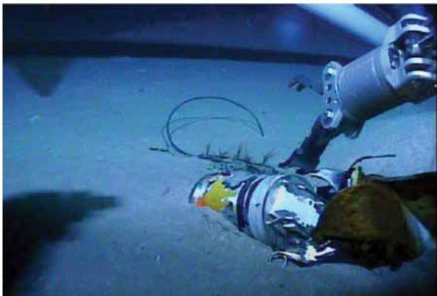
Remote operating vehicle (ROV) manipulator arm positioned above the EL FARO S-VDR capsule on the sea floor prior to the capsule recovery
