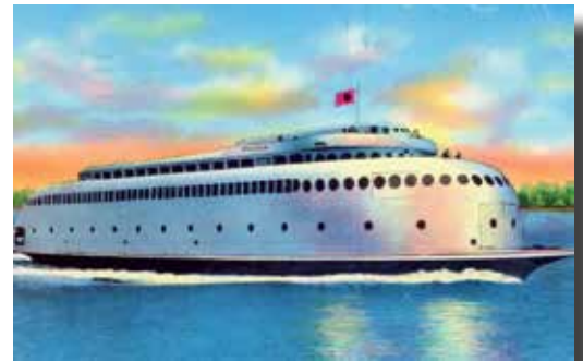
The Kalakala: On her Maiden Voyage from Seattle to Bremerton on July 3, 1935, Under the management of the Black Ball Line she had 500 guests on board and 100,000 spectators crowded around Coleman Dock. Billed as "Unsinkable" with eight watertight bulkheads. Ship particulars: 276 LOA, 55 ft, 8 in W, Speed -18 knots, Capacity 2,000 passengers.
