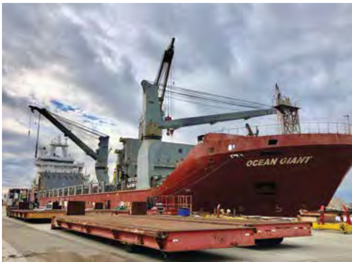
MSC chartered ship, MV Ocean Giant , loads sections of the Marine Causeway System in Port Hueneme, CA. The steel sections will be married together on location at the McMurdo Station to create a pier for discharging and loading cargo at the station.
