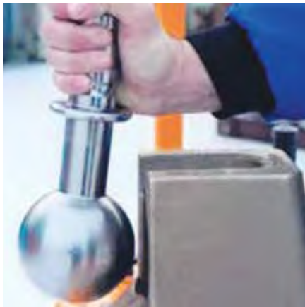
32 Single hook for use with a single fall & hook system on lifeboats.
