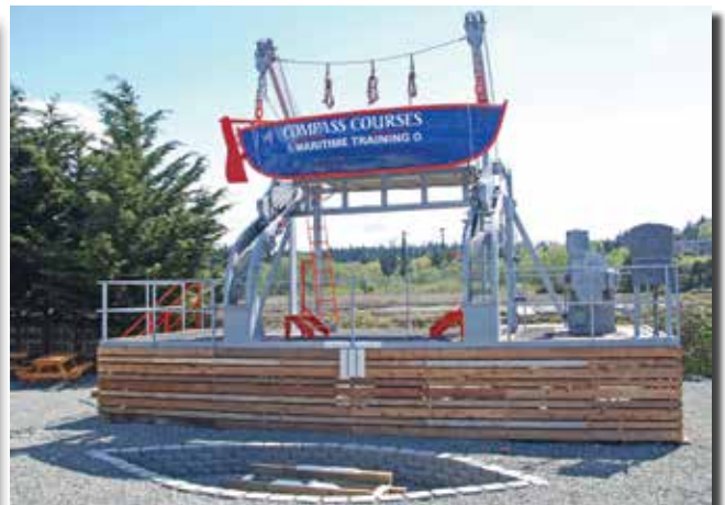
The Pride of Compass Courses. Their own portable gravity lifeboat davit. This allows for hands on training for future mariners.
