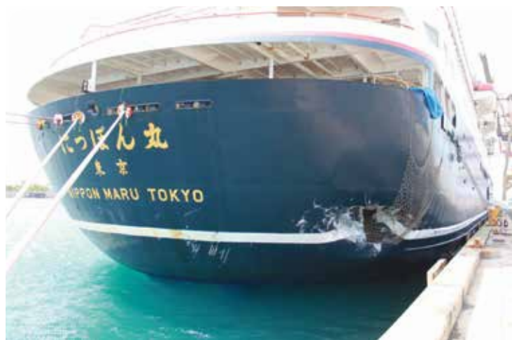
Damage to the stern of the Nippon Maru
