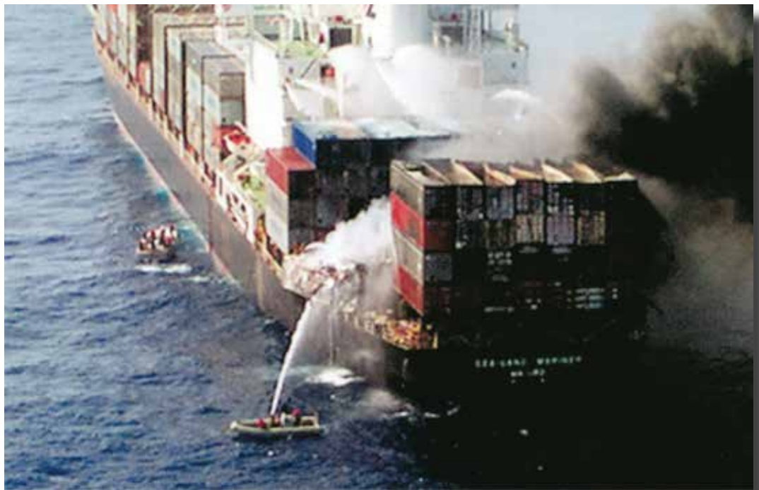
Ship's fixed monitors were used to subdue a fire aboard the Sea-Land Mariner, which was built in 1980. The fire occurred in April 1998 as a result of an explosion caused by mislabeled class 9 hazardous cargo and was brought under control by the ship and the USS Wasp. Note the difference in water pressure exerted by the monitors compared to that of the fire hoses used on the APL Vancouver.
