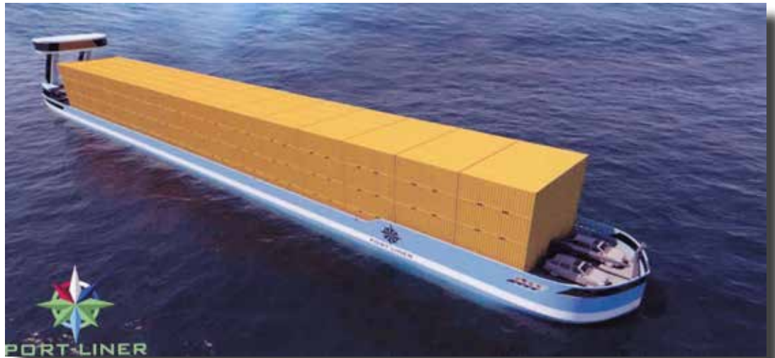
Port Liner's all electric barge – note the two trucks on the bow.
