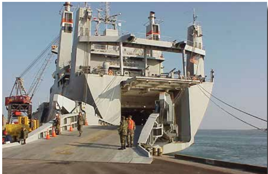
The MV Cape Trinity preparing to load vehicles through her stern ramp. The Ro-Ro ship was built in 1977 and her hull is ice strengthened. She is an ROS-5 status ship, meaning she is able to be activated and ready for service in 5 days. The Capt Trinity (T-AKA-9711) is part of MARAD's Ready Reserve Force at Beaumont, TX.
