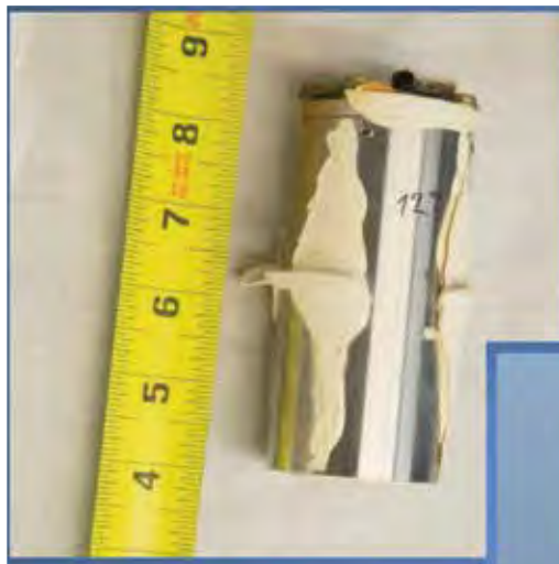
Internal cylinder and digital circuit board of the El Faro's Voyage Data Recorder
