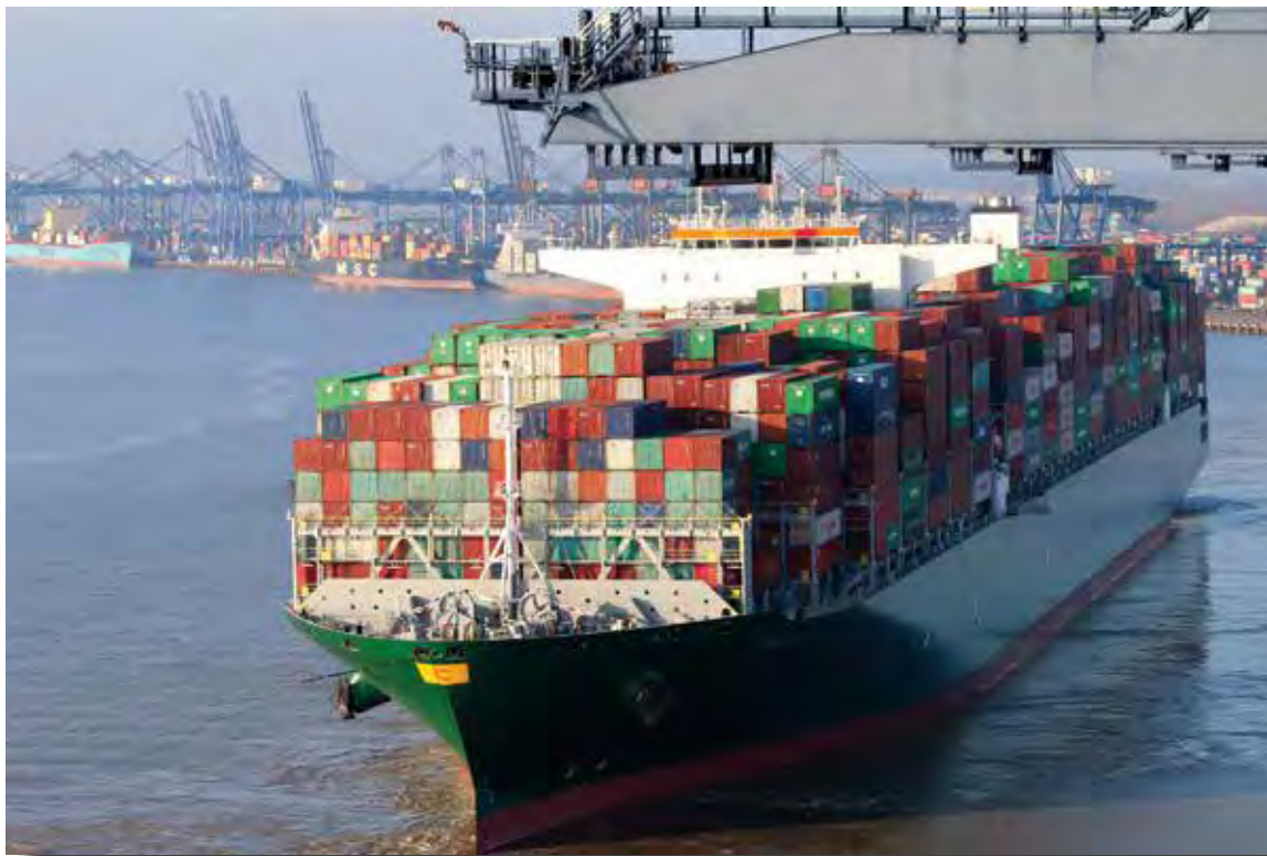
An Evergreen VLCS coming alongside. VLCS (Very Large Container Ship) is one with a capacity of 10,000 to 14,500 TEUs. An ULCS (Ultra Large Container Ships) has a capacity greater than 14,500 TEUs.
