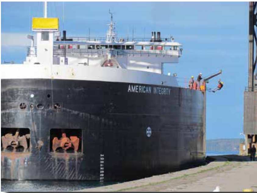
A deckhand is lowered to the pier as the American Integrity prepares to enter the Poe Lock. On the Great Lakes the "line handlers" are supplied by the ship's crew.
