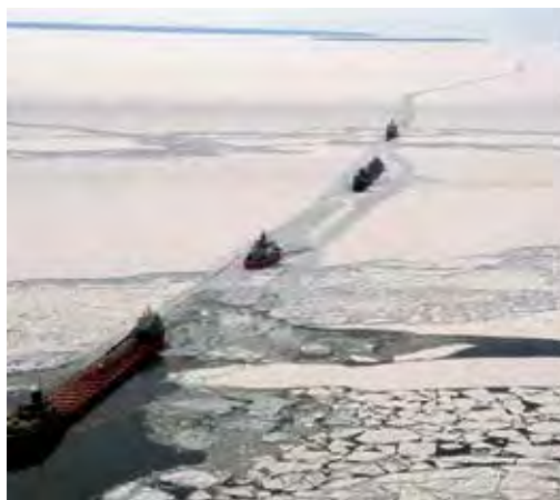
The Coast Guard Cutter Mackinaw, and the Canadian Coast Guard Ship Pierre Radisson, conduct an escort on Lake Superior near Whitefish Point April 3, 2014. Worked together they were able to break sheet ice nearly 40 inches thick.
