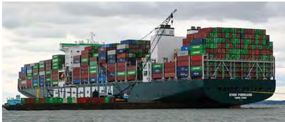
View from the port quarter of Ever Forward, aground east of the Craighill Channel. On April 17, 2022 at approximately 0700, the Ever Forward was successfully pulled back into the channel and refloated, after dredging 206,280 cubic yards of material and the removal of 505 containers.
