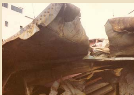
Above: Main deck and gunwale angle bar, heavy damage. Center: Sideshell, in way of No's 3 and 4 holds, opened up. Right: No. 4 clean up of oil, potash and sea water underway.
