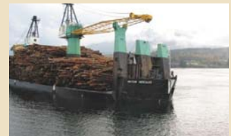
RIVTOW HERCULES pre-flooded and ready to start tipping procedure.
