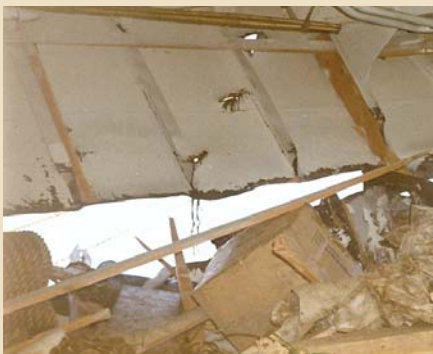
Above: Under Foc's'le head, store, port side, looking forward. Center: bow and forefoot set over to starboard. Right: lower portion of frames torn and internals buckled.
