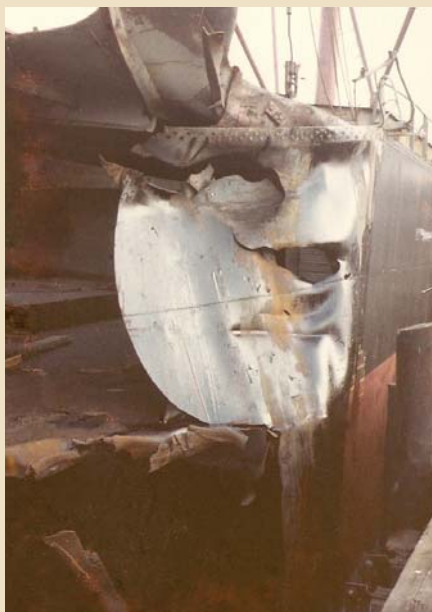
Above: Main deck and gunwale angle bar, heavy damage. Center: Sideshell, in way of No's 3 and 4 holds, opened up. Right: No. 4 clean up of oil, potash and sea water underway.
