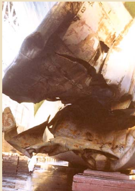
Above: Under Foc's'le head, store, port side, looking forward. Center: bow and forefoot set over to starboard. Right: lower portion of frames torn and internals buckled.
