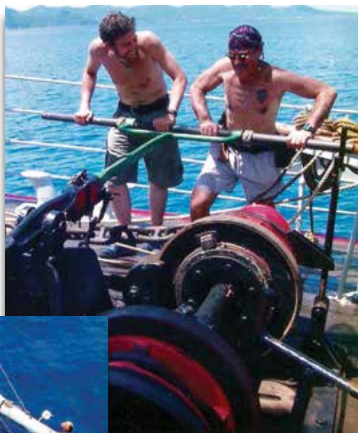
Above: Working the anchor windlass (one cycle puts the chain up one link.)
