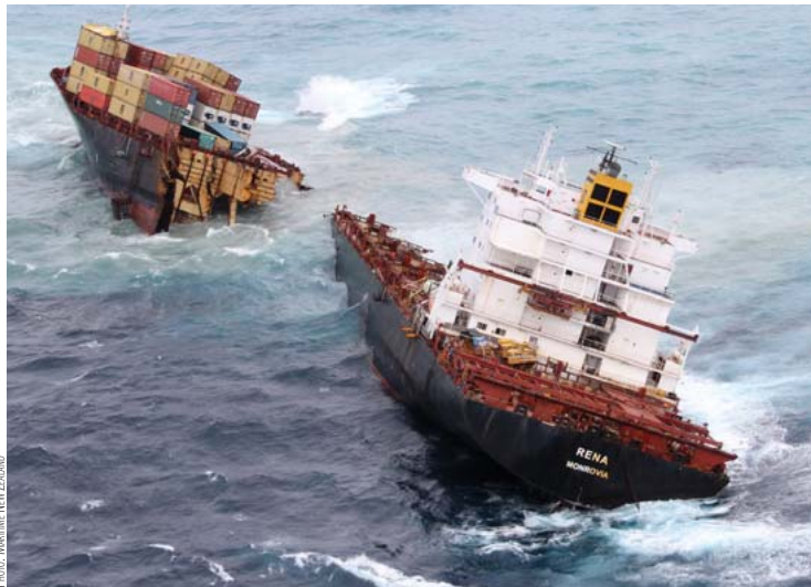
Above: Aerial shot taken January 8, 2012. RENA separated into two pieces after being battered by 6m waves the previous night.
