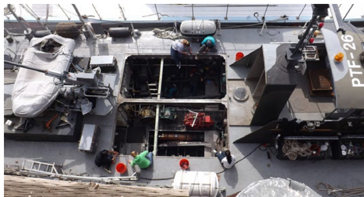
Above: LIBERTY crew prepares softpatch combing during main engine swap. Right, top: Captain Klaus Niem present Captain Jim West with a donation to the Liberty Maritime Museum Sea Scouts program. Right, middle: LIBERTY crew prior to dress inspection onboard HORNET . Right, bottom: LIBERTY , after Old Salts Regatta, 2012.
