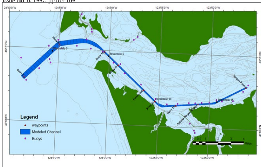
Figure 3. Arrangement of the DUKC ® calculation locations for the Columbia River Bar. Calculation locations are arranged every ¼ mile (400 m) along the deep-draft shipping channel. This layout provides sufficient resolution to capture spatial variation in ship keel elevation while keeping computational effort to a manageable level.
