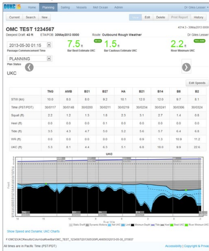
Figure 5. Example output of the demonstration DUKC® system showing a profile of UKC-related information for a particular transit of a specific ship. Black indicates sea bed, light grey is ship’s draft and dark grey is dynamic motions allowance. Pale blue indicates predicted UKC.
