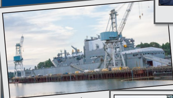
VIGOROUS, the largest floating drydock in the U.S. with a lifting capacity of 80,000 LT, inside width 186 feet and length 960 feet.
