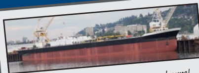
578-foot ATB with a 185,000-barrel carrying capacity for Kirby Maritime, built by Gunderson Marine.
