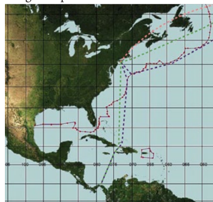
Red dotted line represents the ECA boundary. Green dash lines are existing routes; purple dash lines denote alternate route course.
