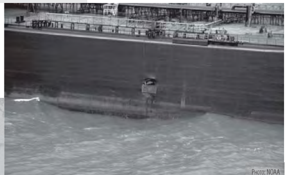
M/V HEBEI SPIRIT damage after a crane barge owned by Samsung collided with the anchored tanker on December 8, 2007.
