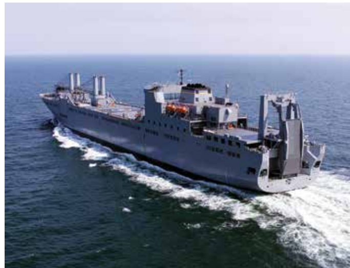
USNS MV Roy P. Benavidez is one of Military Sealift Command's nineteen Large, Medium-Speed Roll-on/Roll-off Ships and is part of the 18 ships in Military Sealift Command's Sealift Program. Length: 950 feet Beam: 106 feet Draft: 34 feet Displacement: 62,069 long tons Speed: 24 knots Civilian: 30 contract mariners The vessel is named after a Congressional Medal of Honor awardee.
