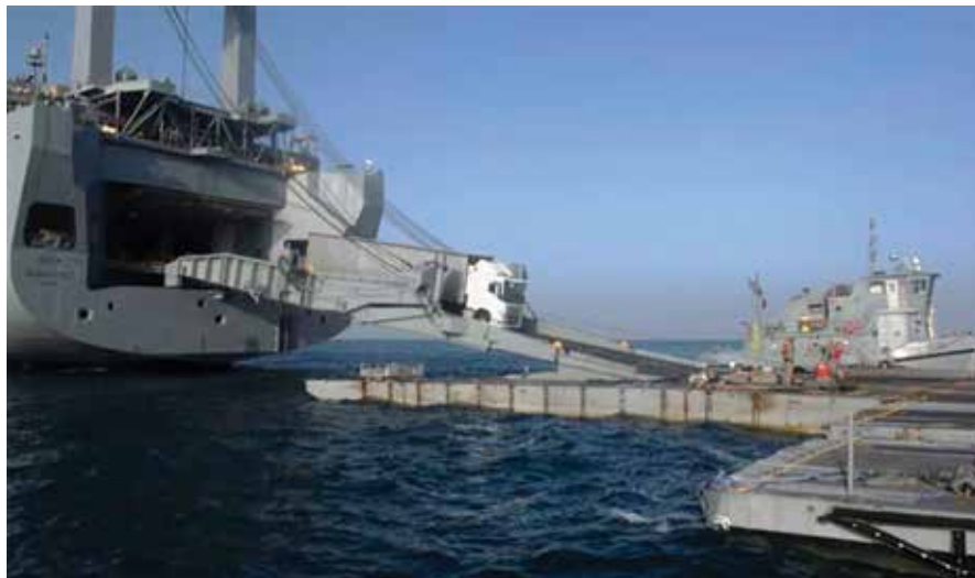
A truck with humanitarian aid drives down the ramp from the MV Roy P. Benavidez (T-AKR 306) onto the Gaza floating dock (roll-on/roll-off discharge facility (RRDF)). The men and women of U.S. Central Command are proud to support USAID in the delivery of humanitarian assistance to Gaza. This corridor is a multinational and combined effort led by USAID and the Department of Defense - alongside the Republic of Cyprus, the United Nations, and international donors, including the UAE, the United Kingdom, Romania, and the European Union.
